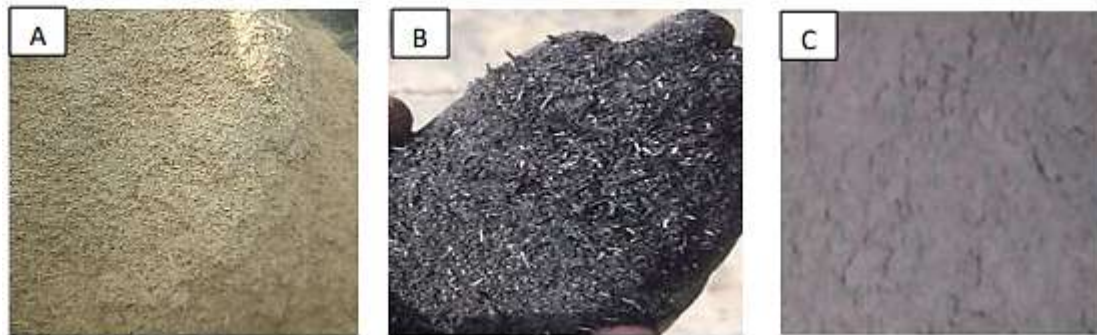
Fig 1:(a) Rice husk before burning (b) Rice husk after burning (c) Rice husk ash
